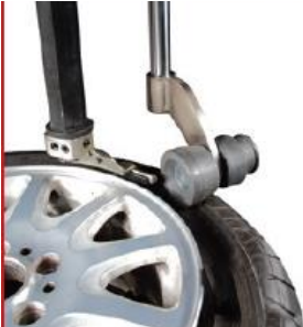
Single point assister arm for helping remount those hard to fit low profile tyres
